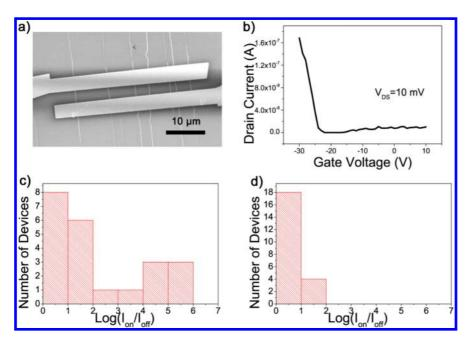
Figure 4. (a) SEM image of a multiple-tube device with a channel length of 2  $\mu$ m. (b) Transfer characteristics of a representative multiple-tube device. (c, d) Histograms of the on/off ratio of each multiple-tube device based on Fe—W-catalyzed (c) and Fe-catalyzed (d) SWNTs under optimized water vapor concentration during growth.
