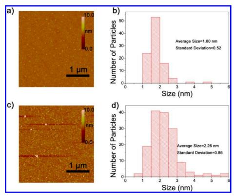
Figure 1. AFM images for Fe-W (a) and Fe (c) nanoparticles on the SiO<sub>2</sub>/Si substrate. Size distributions for Fe-W (b) and Fe (d) nanoparticles after CVD growth for 15 min at 900  $^{\circ}$ C. Over 100 particles were measured for each sample.
